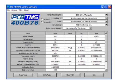
manufacturer defined templates. Principle types of transducers supported are accelerometers, microphones, charge amplifiers, and microphone preamplifiers. A triaxial adapter (optional) is available for direct interface with triaxial accelerometers with one mouse-click.
